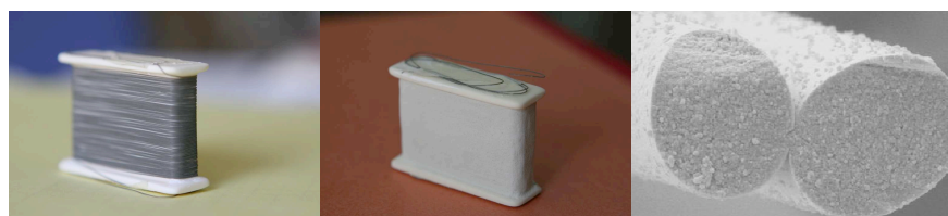
Fig. 2 – Rectangular coil prototype (NSTX design): initial winding, MgO wrapping, and detail of the 2D reinforcing material in Alumina Nextel 610.
