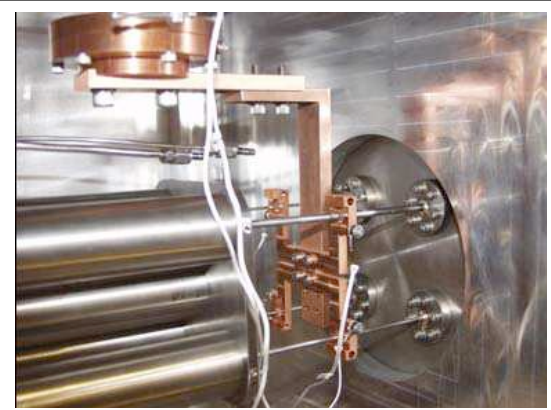
Figure 3. The pellet injector cavity built at O.R.N.L.
