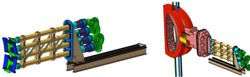
Fig.4. ICRH Antenna System (CATIA 3D Model)
