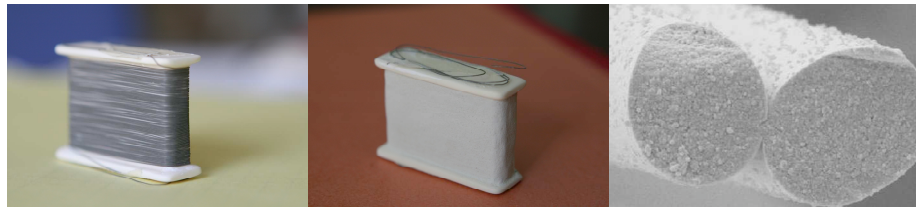
FIGURE 1. Rectangular coil prototype (NSTX design): initial winding, MgO wrapping, and detail of the 2D reinforcing material in Alumina Nextel 610.
