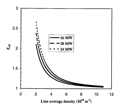
Fig 2. Degree of plasma contamination as a function of density according to the scaling of Ref.[5] applied to Ignitor, for different amounts of radiated power.
