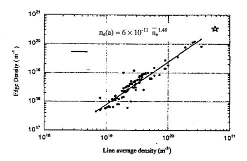
Fig. 4. Experimental values of the edge density vs the line average density. The star represents the extrapolated value for the reference Ignitor discharge.
