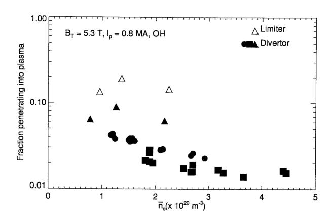
Fig 1. Effect of electron density on the plasma screening of Ar impurity ions in experiments by the Alcator C-Mod machine.
