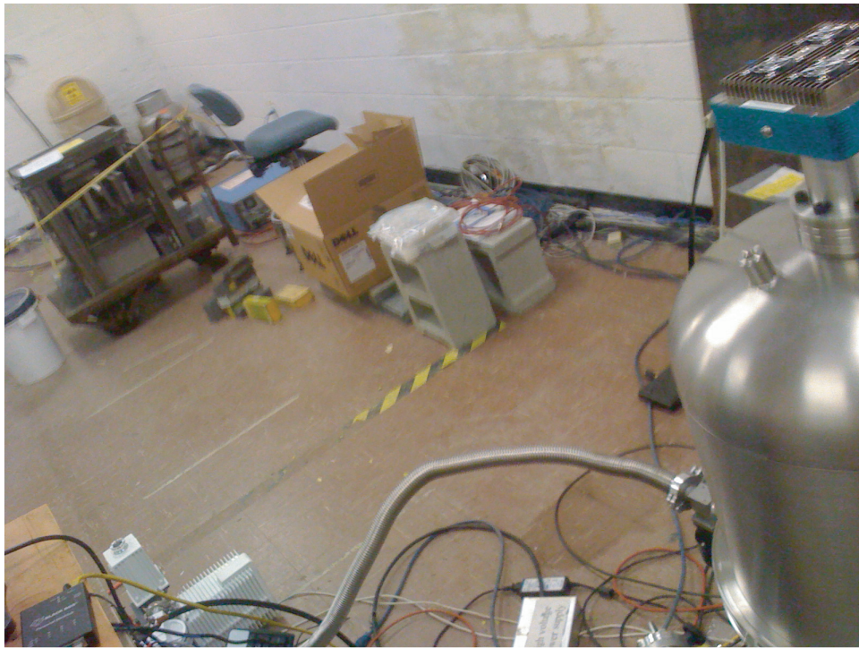
Figure 3: Lab setup. The detector is in the foreground right and the source is located inside the neutron shielding on the cart on the extreme left of the picture. The distance from the source to the center of the detector is 4 m.
