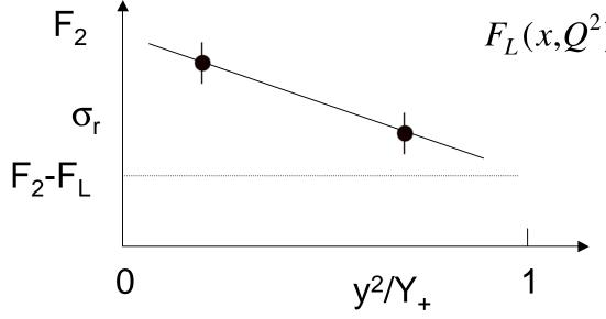
$$F_L(x,Q^2) = \frac{\sigma_r(x,Q^2,y_1) - \sigma_r(x,Q^2,y_2)}{f(y_2) - f(y_1)}$$
