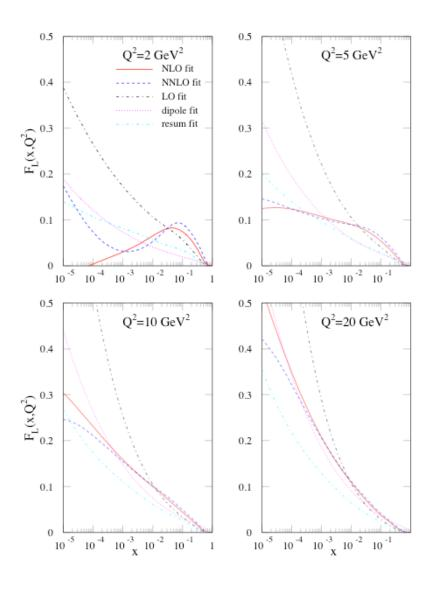
$F_L$  predictions from MRST group at different orders in DGLAP, a fit which resums the leading  $\ln(1/x)$  and  $\beta_0$  terms, and a dipole type model. Very large differences at small  $Q^2$  where gluon uncertainty large.
